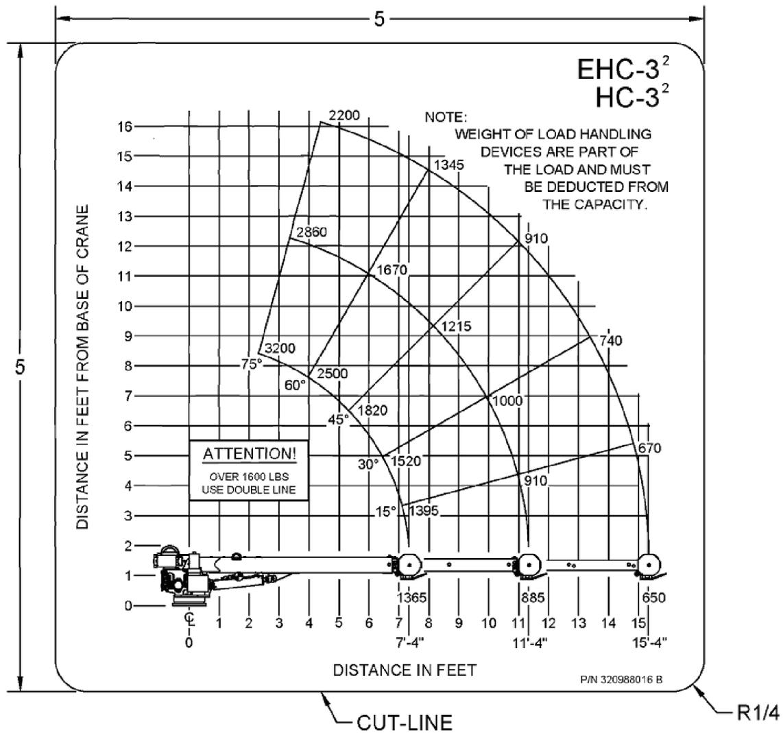
**Note: Max lifting capacity is 3,200 lbs.**
