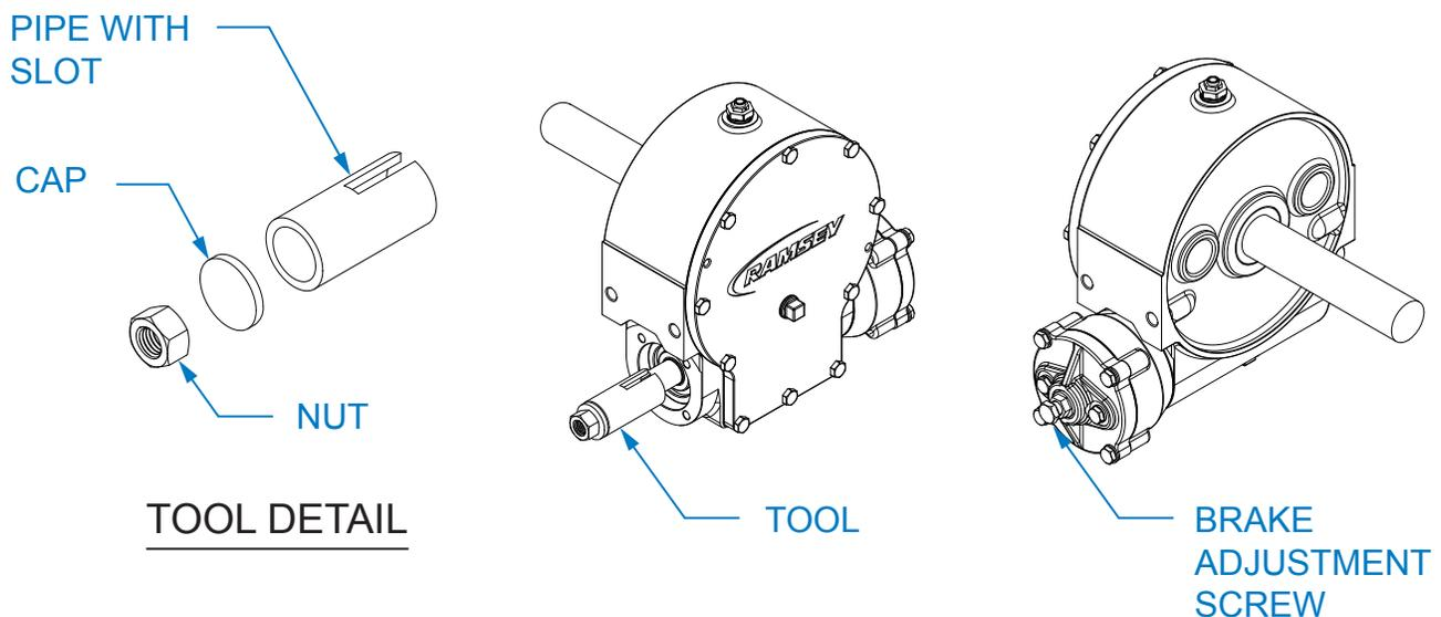
After welding the cap and nut to the tubing, slot the tubing as shown. This will allow the special adapter to slide over the keyway and then act as a large socket. A torque wrench can then be used to apply the proper torque. Turn the torque wrench so that the drum turns in the spool out direction or lowering direction. The torque ratings should be between 8-13 ft-lbs.
