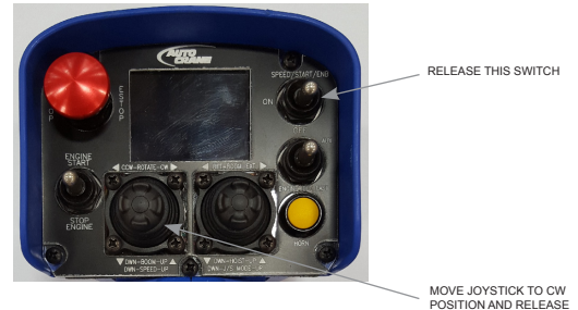
Figure 3—LCD screen display & transmitter during step 3
